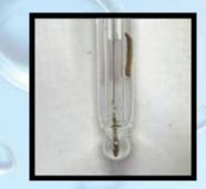
Never wipe the glass membrane because it can lead to permanent damage! DO NOT BE ALARMED IF ANY SALT DEPOSITS ARE PRESENT. This is normal with electrodes and they will disappear when rinsed with water.
